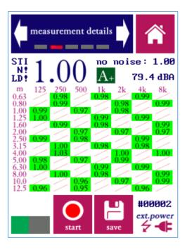
Figure 5. Full STI implementation on the Bedrock SMxx, while measuring. The analyser is synchronized and in the second stage of the signal.
